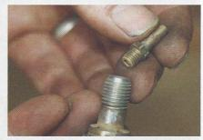
3 Alternative needle jet sizes are simply screwed into the holder. Now, how will different size jets feel on the road?
