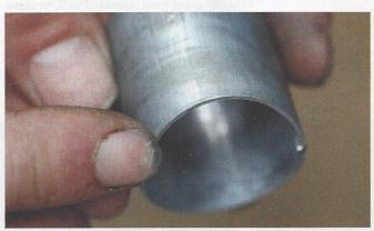
2 This number 3 slide should have a cutaway <sup>3</sup>/<sub>16</sub>in high at its peak. It's worth checking old slides in case they've been modified. When fitting, be sure to locate the guide strip on the inside diameter with the corresponding notch in the jet block
