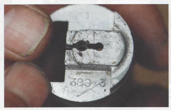
1 The carburettor size and slide cutaway are stamped on the top. Quite logically '389 3' means a '3' cutaway for type 389 carb
