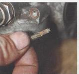
3 Size is stamped on the shank. Witness marks show that the jet's tapered nose has properly sealed in the hole
