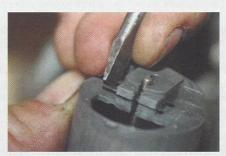
2 ...spring slide and needle retaining clip. Before you remove the latter, make a note of which groove it's in
