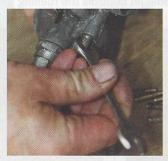
To access the jet, remove the chrome-plated cap nut using a 1/8W spanner. The jet may come out with it but should stay in the carb
