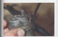
To get at the needle you'll need to first get in by removing the top ring and cap, exposing the...
