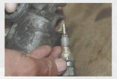
Whipping out the needle jet holder at the bottom of the carb to reveal the needle jet itself
