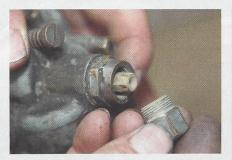
2 Swapping main jets is as simple as removing the cap nut on the bottom of the carburettor...
