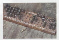
1 You can't play around with main jet sizes if you don't have any alternatives. A set of jets is worth picking up at an autojumble
