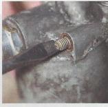
2 There's a screwdriver slot in the end for removal and replacement. Make sure you use a well-fitting screwdriver as the slot is easy to chew up
