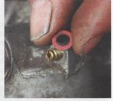
4 Screw the jet home and nip it to seat the taper. Fit a new fibre washer if necessary and replace the plated cap nut
