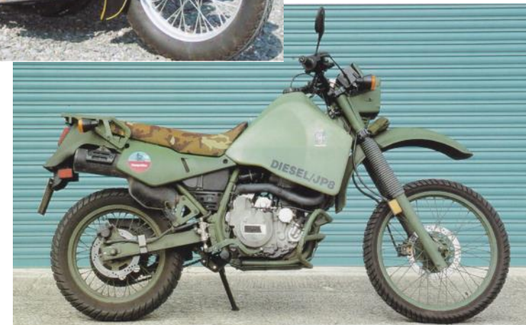
1990 RMCS/Hayes M1030 diesel motorcycle based on the Kawasaki KLR 250
