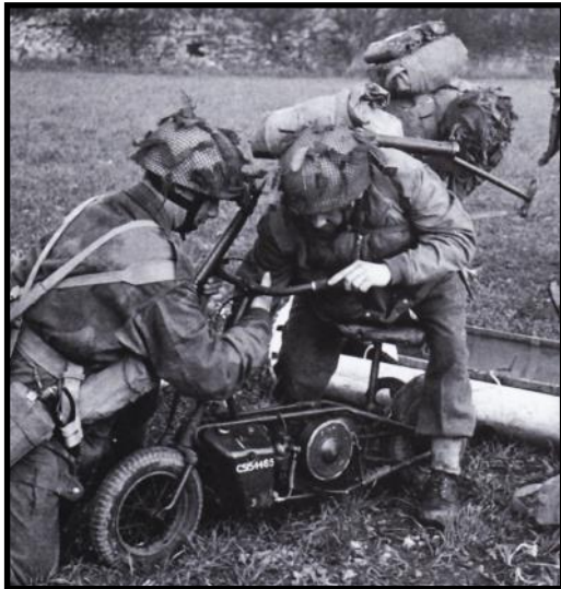
1942-45 Excelsior Welbike 'Parascooter' the smallest military motorcycle. Paras unpack and assemble a Welbike which had been air-dropped in a container. The bike had a post-war life as the 'Corgi' scooter.
