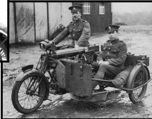
British Clyno/Vickers outfit fitted with a water cooled machine gun and armoured shield WW 1.
