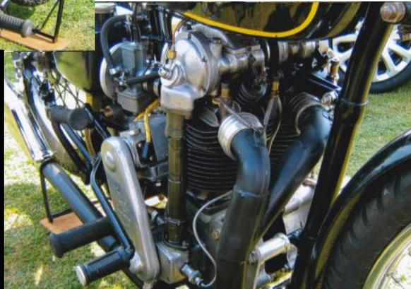
he had built it out of two 250 KSS engines and from start to getting it on the road took about 20 years. Colin bought the parts in the 1940s and 1950s and installed the engine in a MAC frame. He has done a fantastic job don't you think?
