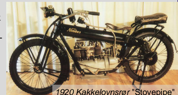
Pressed metal handlebars & instrument panel
