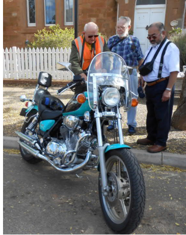
Above Left Roger O'Loughlin's Suzuki 650. He has enlarged the tank capacity by 5 litres for increased range.
